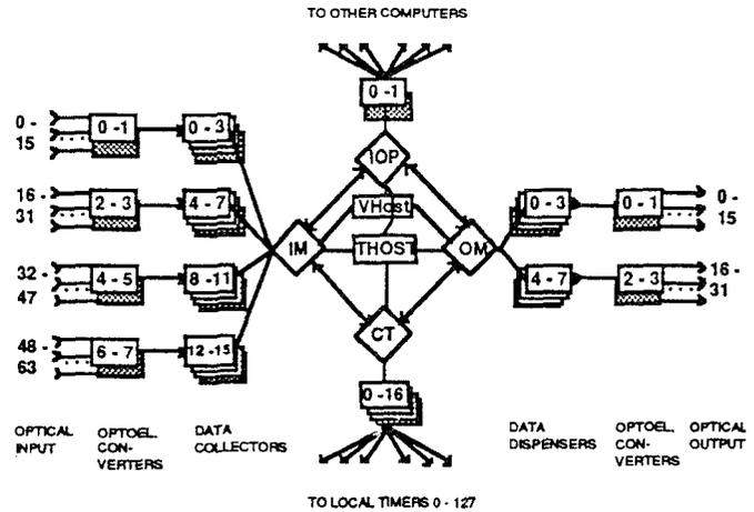
Fig. 2: Block diagram of the feed forward computer. Shown are the transputer- and VMEbus host (THOST, VHOST), input and output master (IM, OM), IOP and central timer (CT), together with the data-collectors and dispensers. More than four links per transputer are made of linkadapters.
