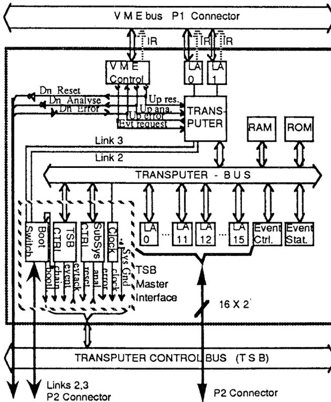
Fig. 4: Block diagram of the MCPU board. LA = fifth link.
