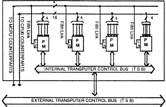
Fig. 5: Block diagram of the CPU0 board. (LA = linkadapter, PM = transputer-memory module).
