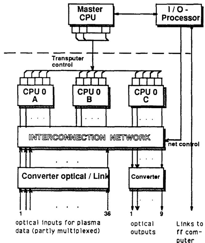
Fig. 8: Architectural block diagram of the feed back computer.
