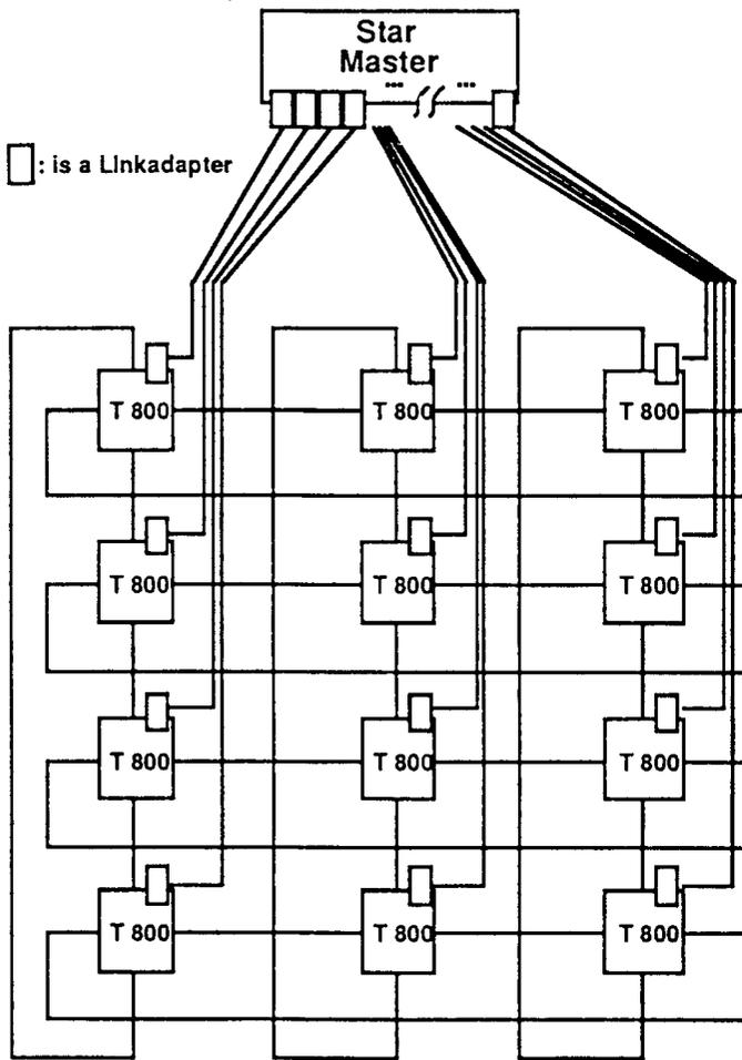
Fig. 9: The Programmers point of view of the feed back computer is a torus with superimposed star topology.
