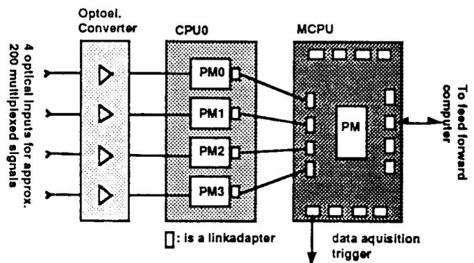
Fig. 10: Block diagram of one monitor computer.
