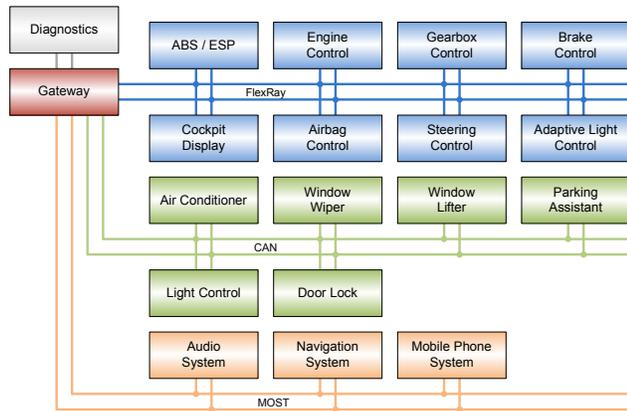
Figure 1. Communication network of a standard vehicle
