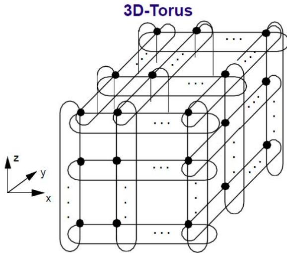
Figure 2. Communication network topology of ConPar
