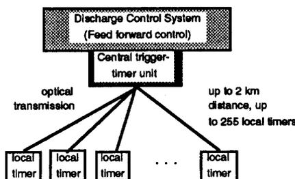
Fig. 1: Physical setup of the trigger-timer system.
