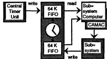
Fig. 6: Protocolling of central timer messages and subsystem output.
