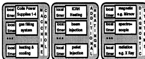
Fig. 2: Unified trigger-timer system for all components of ASDEX-Upgrade.
