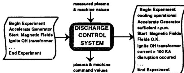
Fig. 4: Merging offline and online and hardware triggered events into one stream of messages to control the tokamak subsystems.
