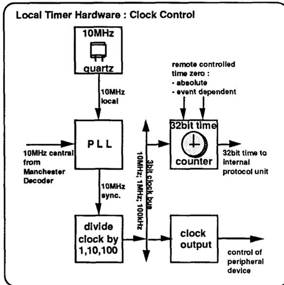
Fig. 9: Block diagram of time reconstruction by local timer.
