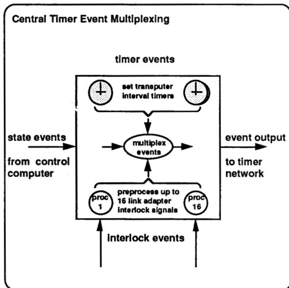
Fig. 4: Block diagram of the central event generation.
