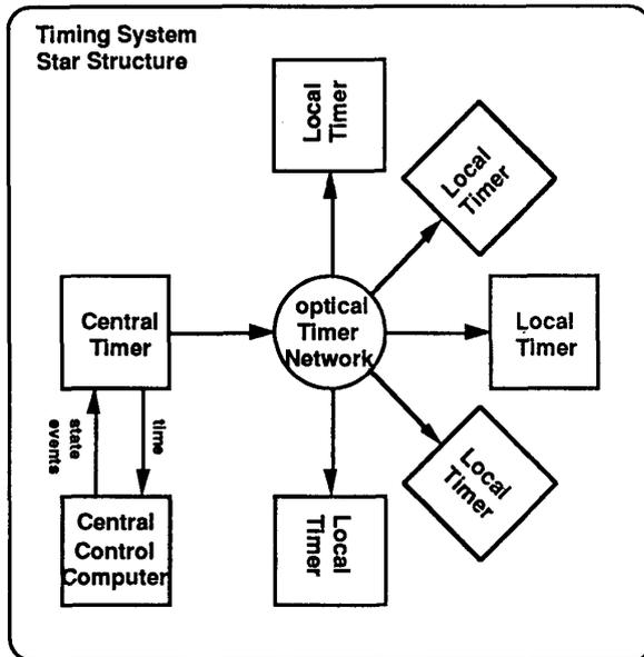
Fig. 2: Structure of the timing system.
