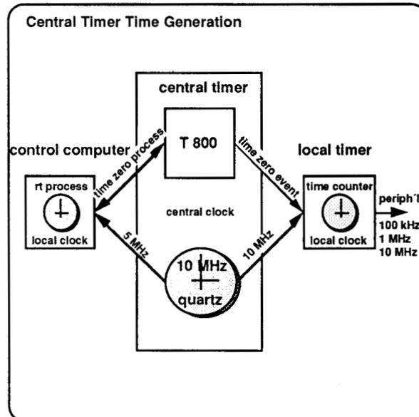
Fig. 5: Block diagram of the central time generation.
