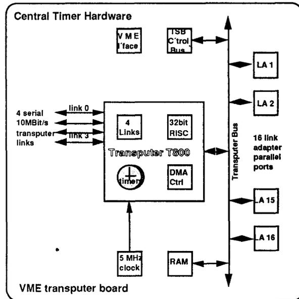
Fig. 3: Block diagram of the central timer VME board.
