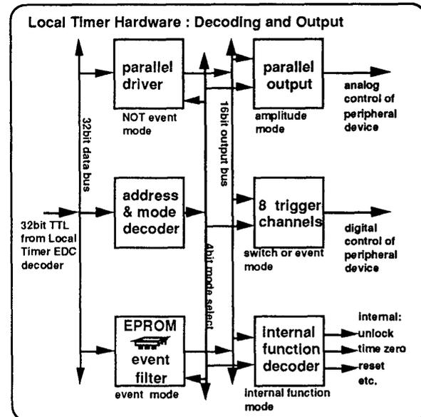
Fig. 10: Block diagram of event decoding and execution.
