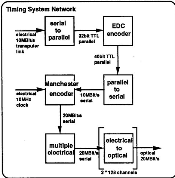
Fig. 6: Block diagram of the the timing networks transmission technique.
