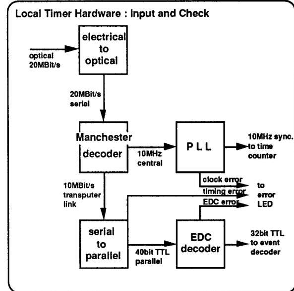
Fig. 8: Block diagram of the local timer input and error checking.
