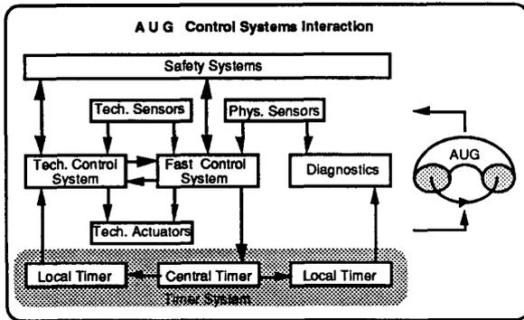
Fig. 1: Structure of the AUG experiment and control system.
