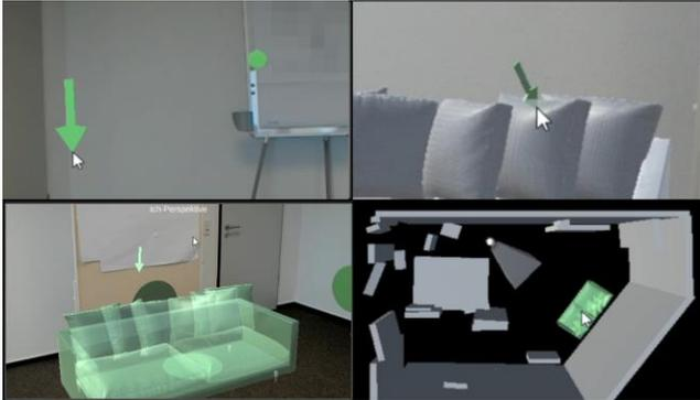
**Figure 1: The different tools tested: Manual Depth Pointer (top left), Assisted Depth Pointer (top right), Manual Depth Egocentric Placement (bottom left), and Assisted Depth Exocentric Placement (bottom right) including the different perspectives taken by consultant (top view, fixed rotation) and client (represented by circle and frustum).**
